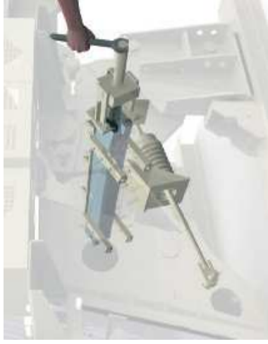
The manual wedge setting adjustment is faster and safer than outdated shim setting adjustment systems.
