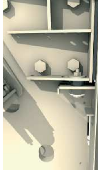
Special rubber dampers and stoppers allow the crusher to move vertically and longitudinally while preventing wear and subsequent damage to the crusher's foundation.
