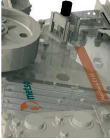
The hydraulic wedge setting adjustment allows you to change the setting in seconds even while the crusher is idling.
